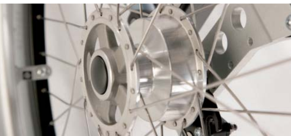
Rear wheel with drum brake system for attendant
