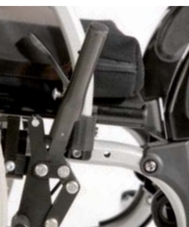
The wheel lock can also be ordered with one-handed operation
