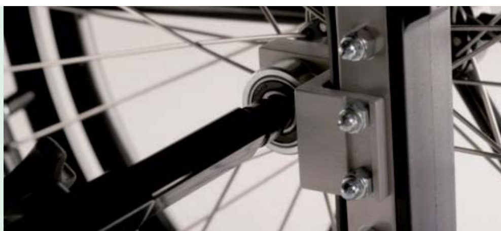
One-arm drive with telescoping axle for independent mobility
