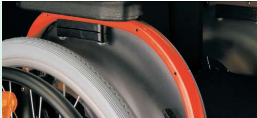
Standard side panel with height adjustment
