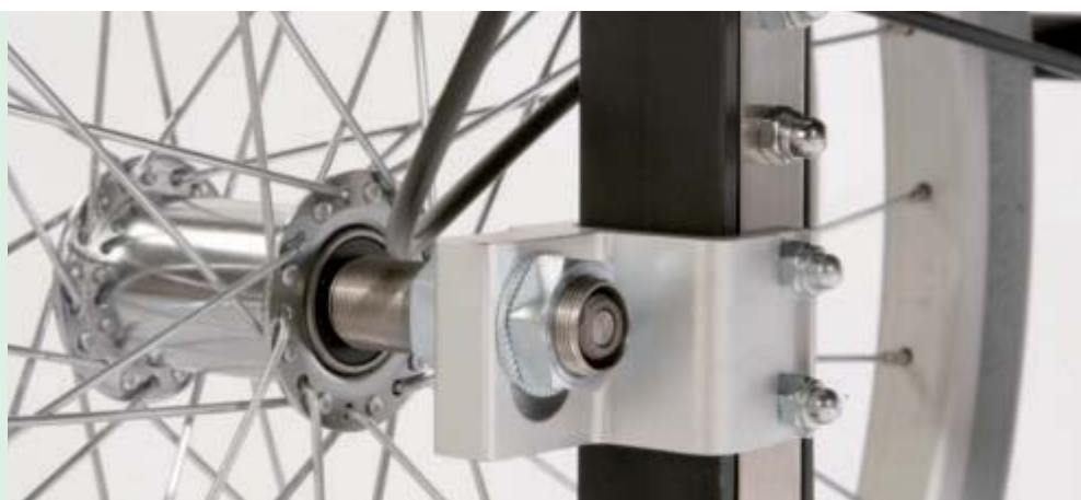
Rear wheels with quick-release axles
